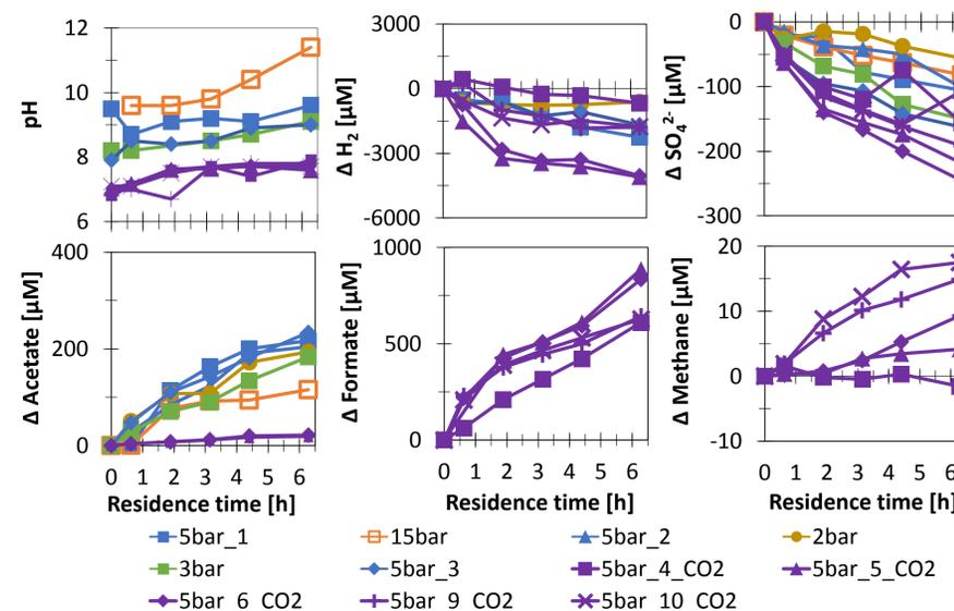
Figure 3. Concentration profiles of pH, hydrogen, sulfate, acetate, formate and methane. Concentrations for all parameters except pH are calculated as delta to the respective inflow concentration. Gas pressure used in each experiment is indicated by the initial number in legend entries (X bar), second number indicates chronological order of profile (5 bar\_X) and "CO<sub>2</sub>" indicates the use of H<sub>2</sub>-CO<sub>2</sub> gas mixture to reduce pH.
