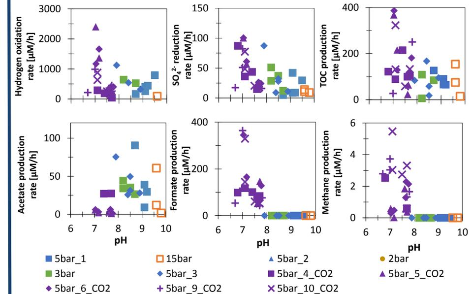
Figure 4. 0<sup>th</sup> order rates, calculated between the column's sampling ports, shown versus the particular pH for processes of hydrogen oxidation, sulfate reduction, formate production and acetogenesis. Gas pressure used in each experiment is indicated by the initial number in legend entries (X bar), second number indicates chronological order of profile (5 bar\_X) and "CO<sub>2</sub>" indicates the use of H<sub>2</sub>-CO<sub>2</sub> gas mixture to reduce pH.
