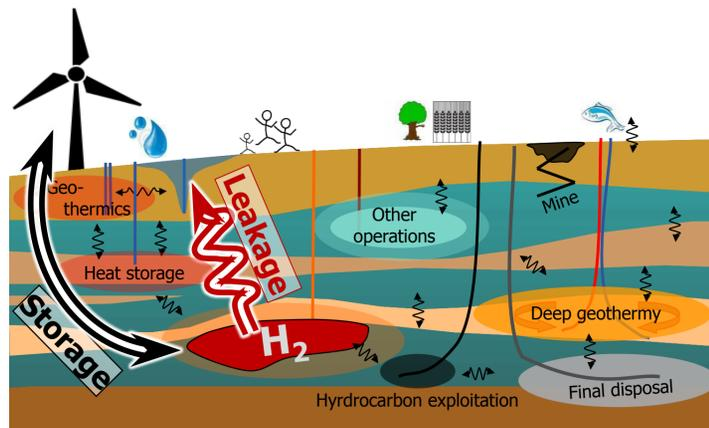
Figure 1. Options and interactions of subsurface energy storage.
